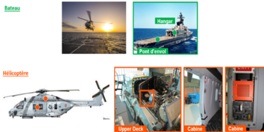
Figure 1 : sensors installation on the ship (hangar/flight deck) and on the Helicopter (upperdeck/cabine)
